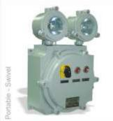
Consist of two units of LED Lamps, automatically switches – **ON**, on mains power failure & provides illumination on battery source for specified duration, after which the battery gets automatically cut-off, to facilitate quick recharge on the resumption of mains supply. Once the battery is fully charged, it automatically slides into trickle charge to constantly retain the charge and be ready for immediate use.
