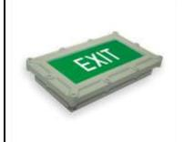
An industrial range of **FLAME PROOF** fitting which, automatically switches – **ON**, on mains power failure & provides illumination on battery source for specified duration, after which the battery gets automatically cut-off, to facilitate quick recharge on the resumption of mains supply. Once the battery is fully charged, it automatically slides into trickle charge to constantly retain the charge and be ready for immediate use.
