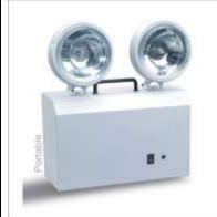
Consist of two 25 Watts Tungsten Halogen lamps, automatically switches – **ON**, on mains power failure & provides illumination on battery source for specified duration, after which the battery gets automatically cut-off, to facilitate quick recharge on the resumption of mains supply. Once the battery is fully charged, it automatically slides into trickle charge to constantly retain the charge and be ready for immediate use.
