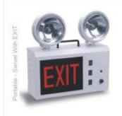
Consist of twin tungsten halogen lamps automatically switches – **ON,** on mains power failure & provides illumination on battery source for specified duration, after which the battery gets automatically cut-off, to facilitate quick recharge on the resumption of mains supply. Once the battery is fully charged, it automatically slides into trickle charge to constantly retain the charge and be ready for immediate use.
