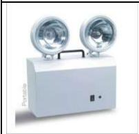
Consist of two 20 Watts Tungsten Halogen lamps, automatically switches – **ON**, on mains power failure & provides illumination on battery source for specified duration, after which the battery gets automatically cut-off, to facilitate quick recharge on the resumption of mains supply. Once the battery is fully charged, it automatically slides into trickle charge to constantly retain the charge and be ready for immediate use.
