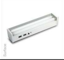
Consist of single or more FT – Ls which provides illumination on normal mains power supply and the same lamp/s continues to provide illumination during mains failure on self contained battery source. **ON** resumption of mains supply, the lamp/s switches back to the mains automatically & simultaneously starts recharging the battery to the required level. **Maintained models provide uninterrupted illumination.**
