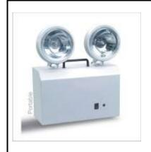
Consist of two 10 Watts Tungsten Halogen lamps, automatically switches – **ON**, on mains power failure & provides illumination on battery source for specified duration, after which the battery gets automatically cut-off, to facilitate quick recharge on the resumption of mains supply. Once the battery is fully charged, it automatically slides into trickle charge to constantly retain the charge and be ready for immediate use.
