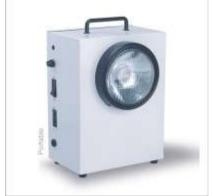
Consist of single 55 Watts incandescent lamp, automatically switches – **ON**, on mains power failure & provides illumination on battery source for specified duration, after which the battery gets automatically cut-off, to facilitate quick recharge on the resumption of mains supply. Once the battery is fully charged, it automatically slides into trickle charge to constantly retain the charge and be ready for immediate use.
