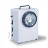
Consist of single 25 Watts incandescent lamp, automatically switches – **ON**, on mains power failure & provides illumination on battery source for specified duration, after which the battery gets automatically cut-off, to facilitate quick recharge on the resumption of mains supply. Once the battery is fully charged, it automatically slides into trickle charge to constantly retain the charge and be ready for immediate use.
