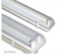
Out door type, consist of single or more FT – Ls which provides illumination on normal mains power supply and the same lamp/s continues to provide illumination during mains failure on self contained battery source. **ON** resumption of mains supply, the lamp/s switches back to the mains automatically & simultaneously starts recharging the battery to the required level. **Non-Maintained models provide uninterrupted illumination.**
