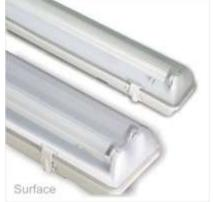
Out door type, consist of single or more FT – Ls which provides illumination on normal mains power supply and the same lamp/s continues to provide illumination during mains failure on self contained battery source. **ON** resumption of mains supply, the lamp/s switches back to the mains automatically & simultaneously starts recharging the battery to the required level. **Maintained models provide uninterrupted illumination.**
