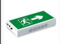
A wall mounting fitting, consist of single CF – L which provides illumination on normal mains power supply and the same lamp/s continues to provide illumination during mains failure on self contained battery source. **ON** resumption of mains supply, the lamp/s switches back to the mains automatically & simultaneously starts recharging the battery to the required level. **Maintained models provide uninterrupted illumination.**
