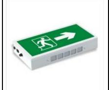
Automatically switches – **ON,** on mains power failure & provides illumination on battery source for specified duration, after which the battery gets automatically cut-off, to facilitate quick recharge on the resumption of mains supply. Once the battery is fully charged, it automatically slides into trickle charge to constantly retain the charge and be ready for immediate use.
