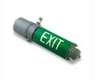
An industrial range of **FLAME PROOF** fitting which, automatically switches – **ON**, on mains power failure & provides illumination on battery source for specified duration, after which the battery gets automatically cut-off, to facilitate quick recharge on the resumption of mains supply. Once the battery is fully charged, it automatically slides into trickle charge to constantly retain the charge and be ready for immediate use.
