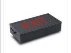
Automatically switches – **ON**, on mains power failure & provides illumination on battery source for specified duration, after which the battery gets automatically cut-off, to facilitate quick recharge on the resumption of mains supply. Once the battery is fully charged, it automatically slides into trickle charge to constantly retain the charge and be ready for immediate use.
