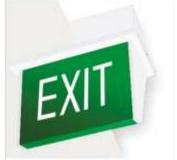
Recessed Mounting Type, single CF - L which provides illumination on normal mains power supply and the same lamp continues to provide illumination during mains failure on self contained battery source. **ON** resumption of mains supply, the lamp switches back to the mains automatically & simultaneously starts recharging the battery to the required level.
