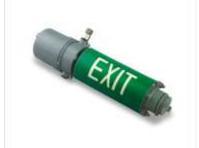
An industrial range of **FLAME PROOF** fitting which, automatically switches – **ON**, on mains power failure & provides illumination on battery source for specified duration, after which the battery gets automatically cut-off, to facilitate quick recharge on the resumption of mains supply. Once the battery is fully charged, it automatically slides into trickle charge to constantly retain the charge and be ready for immediate use.
