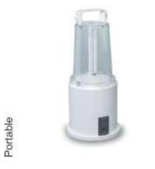
Automatically switches – **ON,** on mains power failure & provides illumination on battery source for specified duration, after which the battery gets automatically cut-off, to facilitate quick recharge on the resumption of mains supply. Once the battery is fully charged, it automatically slides into trickle charge to constantly retain the charge and be ready for immediate use.
