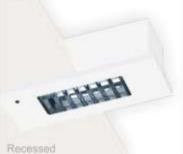
Recess mounting fitting, consist of single FT – L which provides illumination on normal mains power supply and the same lamp/s continues to provide illumination during mains failure on self contained battery source. **ON** resumption of mains supply, the lamp/s switches back to the mains automatically & simultaneously starts recharging the battery to the required level. **Maintained models provide uninterrupted illumination**.
