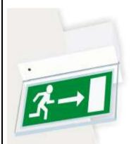
Recessed Mounting Type, single CF - L which provides illumination on normal mains power supply and the same lamp continues to provide illumination during mains failure on self contained battery source.  $\bf ON$  resumption of mains supply, the lamp switches back to the mains automatically & simultaneously starts recharging the battery to the required level.
