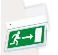
Recessed Mounting Type, single FT – L/CF – L which provides illumination on normal mains power supply and the same lamp continues to provide illumination during mains failure on self contained battery source. **ON** resumption of mains supply, the lamp switches back to the mains automatically & simultaneously starts recharging the battery to the required level. **Maintained models provide uninterrupted illumination.**
