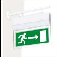
Surface mounting Type, single FT – L/CF – L which provides illumination on normal mains power supply and the same lamp continues to provide illumination during mains failure on self contained battery source. **ON** resumption of mains supply, the lamp switches back to the mains automatically & simultaneously starts recharging the battery to the required level. **Maintained models provide uninterrupted illumination.**
