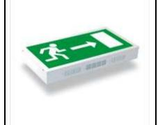
Automatically switches – **ON,** on mains power failure & provides illumination on battery source for specified duration, after which the battery gets automatically cut-off, to facilitate quick recharge on the resumption of mains supply. Once the battery is fully charged, it automatically slides into trickle charge to constantly retain the charge and be ready for immediate use.
