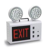
Consist of twin units of LED lamps automatically switches – **ON,** on mains power failure & provides illumination on battery source for specified duration, after which the battery gets automatically cut-off, to facilitate quick recharge on the resumption of mains supply. Once the battery is fully charged, it automatically slides into trickle charge to constantly retain the charge and be ready for immediate use.
