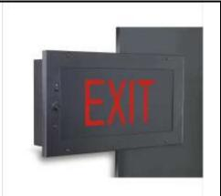
A wall recess mounting fitting, automatically switches – **ON**, on mains power failure & provides illumination on battery source for specified duration, after which the battery gets automatically cut-off, to facilitate quick recharge on the resumption of mains supply. Once the battery is fully charged, it automatically slides into trickle charge to constantly retain the charge and be ready for immediate use.
