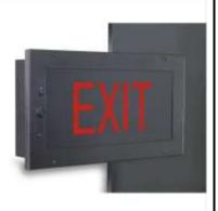
A wall recess mounting fitting, automatically switches – **ON,** on mains power failure & provides illumination on battery source for specified duration, after which the battery gets automatically cut-off, to facilitate quick recharge on the resumption of mains supply. Once the battery is fully charged, it automatically slides into trickle charge to constantly retain the charge and be ready for immediate use.
