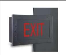
A wall recess mounting fitting, automatically switches – **ON**, on mains power failure & provides illumination on battery source for specified duration, after which the battery gets automatically cut-off, to facilitate quick recharge on the resumption of mains supply. Once the battery is fully charged, it automatically slides into trickle charge to constantly retain the charge and be ready for immediate use.
