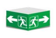
A wall mounting fitting, consist of single FT – L which provides illumination on normal mains power supply and the same lamp/s continues to provide illumination during mains failure on self contained battery source. **ON** resumption of mains supply, the lamp/s switches back to the mains automatically & simultaneously starts recharging the battery to the required level. **Non- Emergency models provide uninterrupted illumination.**
