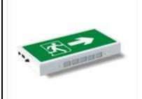
A wall mounting fitting, consist of single FT – L which provides illumination on normal mains power supply and the same lamp/s continues to provide illumination during mains failure on self contained battery source. **ON** resumption of mains supply, the lamp/s switches back to the mains automatically & simultaneously starts recharging the battery to the required level. **Maintained models provide uninterrupted illumination.**
