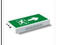
A wall mounting fitting, consist of single FT – L which provides illumination on normal mains power supply and the same lamp/s continues to provide illumination during mains failure on self contained battery source. **ON** resumption of mains supply, the lamp/s switches back to the mains automatically & simultaneously starts recharging the battery to the required level. **Non- Maintained models provide uninterrupted illumination.**
