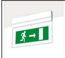
Surface mounting Type, single FT - L which provides illumination on normal mains power supply and the same lamp continues to provide illumination during mains failure on self contained battery source. **ON** resumption of mains supply, the lamp switches back to the mains automatically & simultaneously starts recharging the battery to the required level. **Maintained models provide uninterrupted illumination.**
