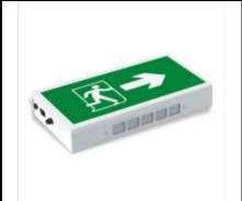
A wall mounting fitting, consist of single CF – L which provides illumination on normal mains power supply and the same lamp/s continues to provide illumination during mains failure on self contained battery source. **ON** resumption of mains supply, the lamp/s switches back to the mains automatically & simultaneously starts recharging the battery to the required level. **Maintained models provide uninterrupted illumination.**
