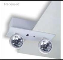
Consist of two 25 Watts Tungsten Halogen lamps, automatically switches – **ON**, on mains power failure & provides illumination on battery source for specified duration, after which the battery gets automatically cut-off, to facilitate quick recharge on the resumption of mains supply. Once the battery is fully charged, it automatically slides into trickle charge to constantly retain the charge and be ready for immediate use.
