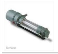
An industrial range of **FLAME PROOF** fitting which, automatically switches – **ON**, on mains power failure & provides illumination on battery source for specified duration, after which the battery gets automatically cut-off, to facilitate quick recharge on the resumption of mains supply. Once the battery is fully charged, it automatically slides into trickle charge to constantly retain the charge and be ready for immediate use.
