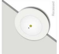
Automatically switches – **ON,** on mains power failure & provides illumination on battery source for specified duration, after which the battery gets automatically cut-off, to facilitate quick recharge on the resumption of mains supply. Once the battery is fully charged, it automatically slides into trickle charge to constantly retain the charge and be ready for immediate use.
