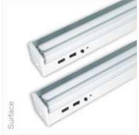
Consist of twin FT – Ls which provides illumination on normal mains power supply and one of the lamps continues to provide illumination during mains failure on self contained battery source. **ON** resumption of mains supply, the lamps switches back to the mains automatically & simultaneously starts recharging the battery to the required level. **Sustained models provide uninterrupted illumination.**
