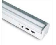
Consist of single or more FT – Ls which provides illumination on normal mains power supply and the same lamp/s continues to provide illumination during mains failure on self contained battery source. **ON** resumption of mains supply, the lamp/s switches back to the mains automatically & simultaneously starts recharging the battery to the required level. **Maintained models provide uninterrupted illumination**.
